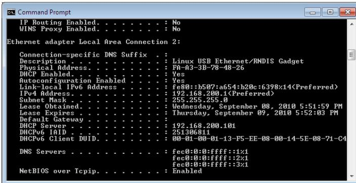
**Figure 24. Command Prompt Window – Adapter IP Address Information**
