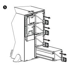
Obsconnect and remove the battery module from the UPS. See "Tower to rack-mount conversion" on page 13.
