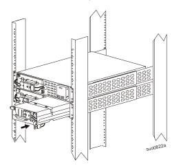
Secure the RBCs to the enclosure. Use three screws on each RBC.
