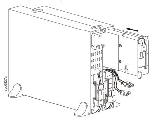
Onnect the two XLBP connectors from the enclosure to the two RBCs. See "XLBP Connectors Installation" on page 6.
