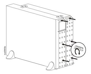
2 Slide the top side battery module into the XLBP.
